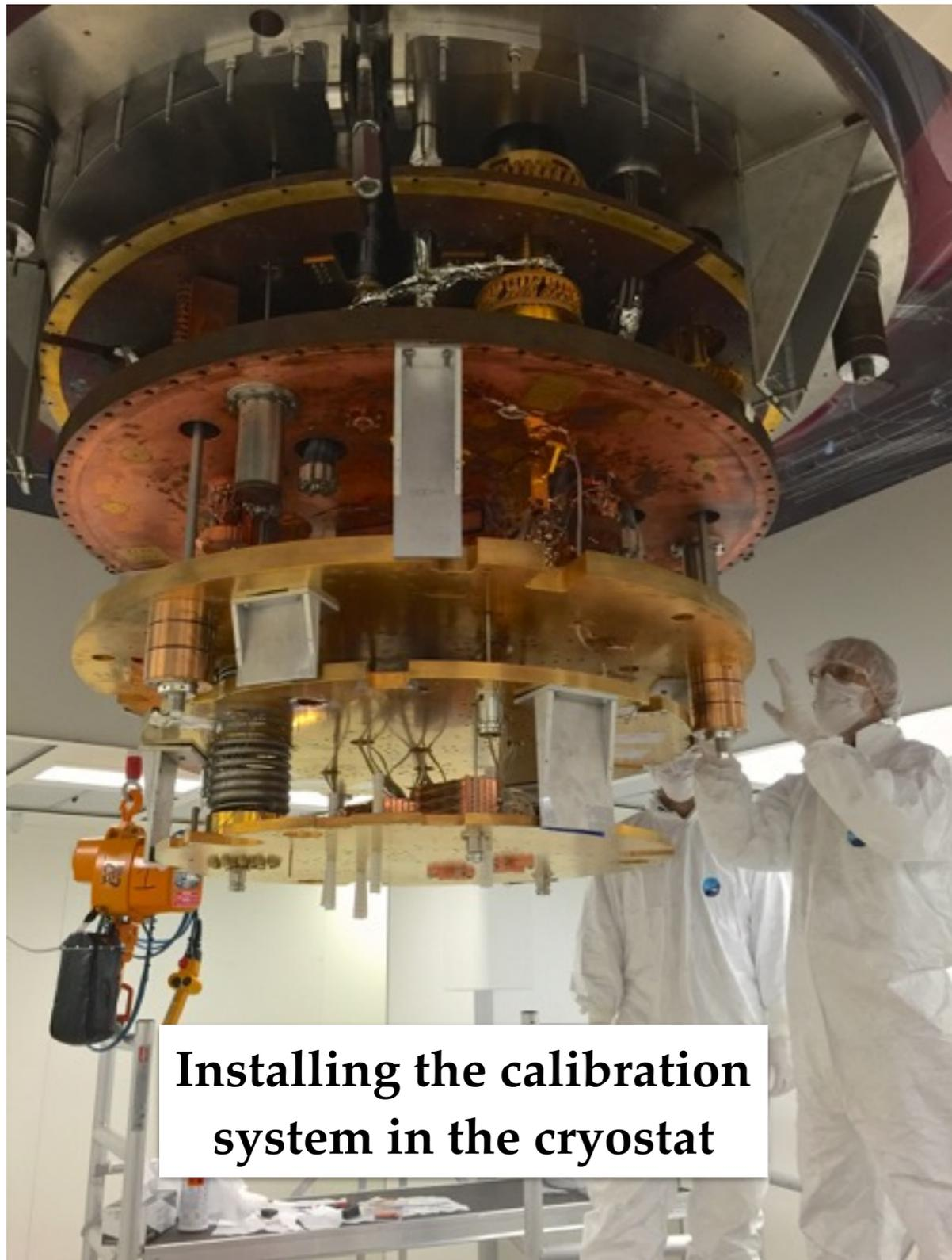
**Installing the calibration system in the cryostat**
