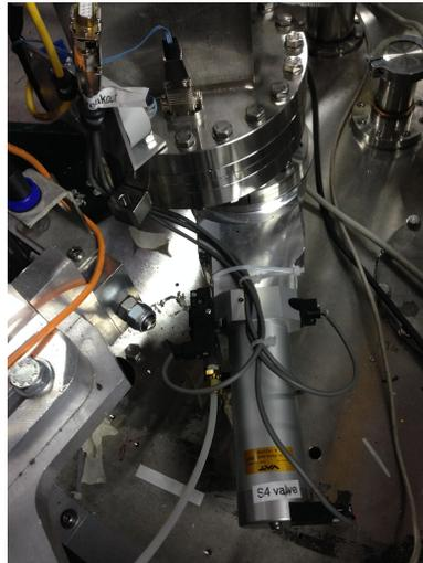
Figure A.36: The cable coming from the motion control box breaks out into the four cables going to the gate valve.
