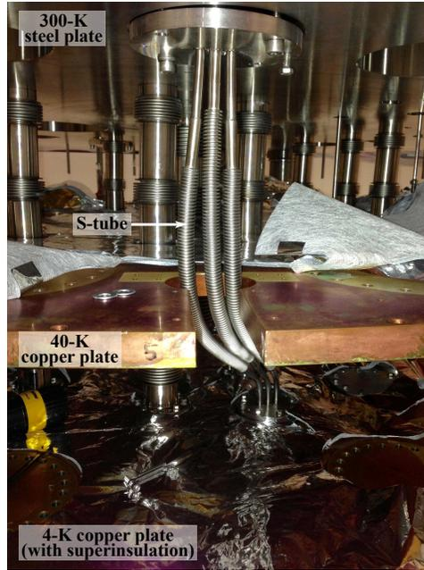
Figure 4.10: An S-tube assembly being installed in the cryostat. Each such assembly contains three string paths and connects the 300-K steel plate (top) to the 4-K copper plate (bottom). The tubes pass through a hole in the 40-K plate, where they are thermalized to the plate with a clamp (not shown).
