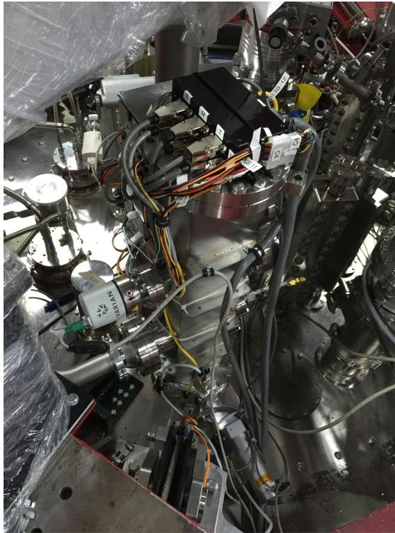
Figure A.27: A photo of the motion box PCB enclosure and wiring.
